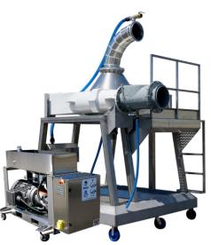
Indoor RAS setup with elevated BP120 skid, auto priming and mobile hydraulic power unit, transfering 4-6kg Atlantic Salmon from growout to purge.
